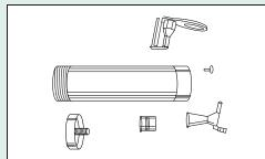
Disassemble items before sterilization in order for the Anprolene gas to penetrate freely.
