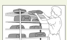
3. Plastic and rubber items should be aerated for an additional 24 hours at 68°F or warmer before use. Metal and glass do not require additional aeration. The room utilized for aeration must have at least ten air changes per hour.
