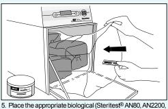
5. Place the appropriate biological (Steritest® AN80, AN2200, AN2203), or chemical indicator (Dosimeter) in the middle of the liner bag. If you cannot verify that the relative humidity is at least 35%, place a Humidichip inside a Humiditube (AN1072) and insert into the liner bag to ensure that the minimum humidity level is met.
