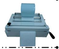
3. The machine will utter "Bi" once when finishing sealing. Using the cutter to divide the pouch from the roll of medical pouch and pulling operating lever up.
