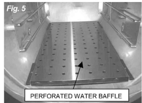
6. Place the Perforated Water Baffle so that it sits on the bottom of the inside of the sterilizer chamber (see Fig. 5).
